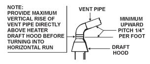
PROPER VENT PIPE INSTALLATION FIGURE 6
